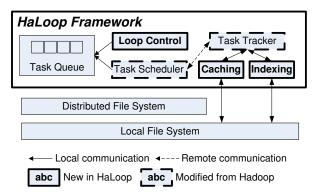
Fig. 6 Overview of the HaLoop framework [22,23].
