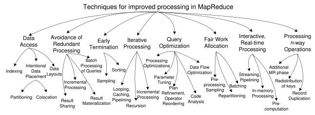
Fig. 3 Taxonomy of MapReduce improvements for efficient query processing.
