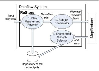
Fig. 5 System architecture of ReStore [40].
