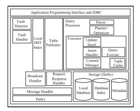
Fig. 1. High-level overview of the architecture of DASCOSA-DB.
