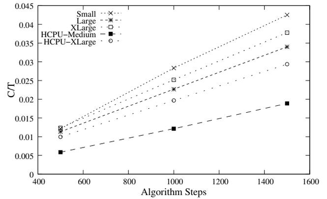
Fig. 5. Values of the C/T metric for AESEncryptDecrypt
