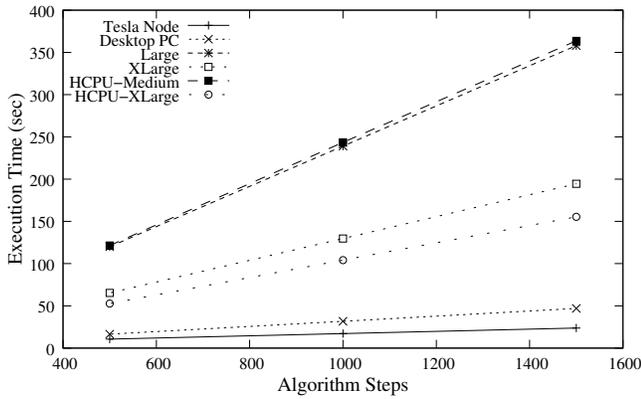
Fig. 2. AESEncryptDecrypt execution times
